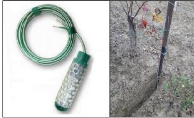
Figure 1 : Installation des sondes Watermark
